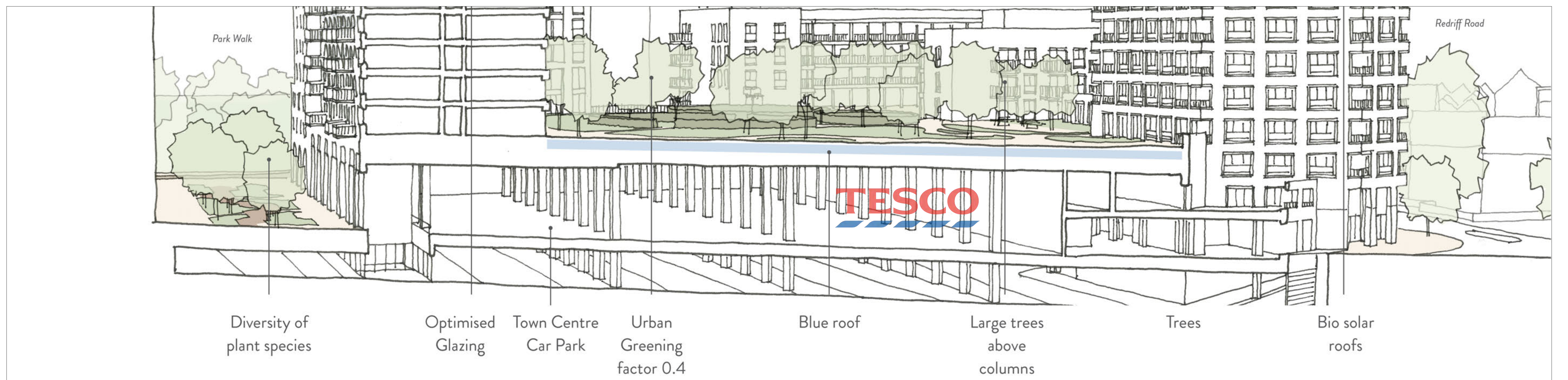
Cross-section of Zone G showing sustainability features included within these proposals
