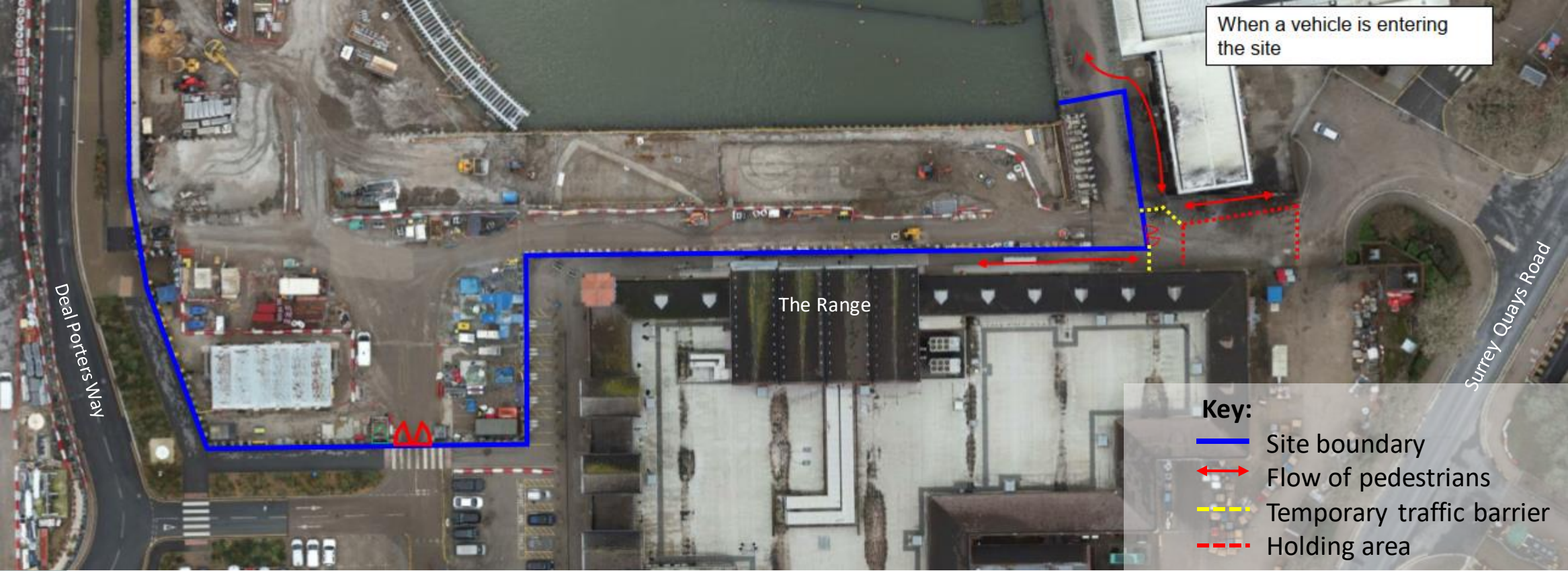
Aerial image of access in southeast corner of the dock when traffic accesses the site
